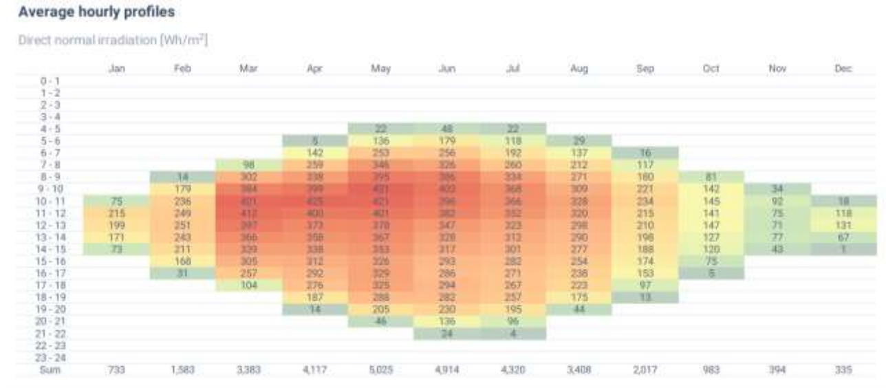
Figure 11. Average hourly profiles of direct normal irradiation in Finland (Wh/m 2 ). Graph from the Global Solar Atlas online app World Bank (2024)
