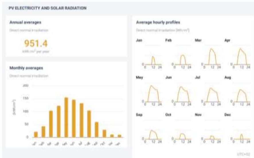
Figure 10. Direct normal radiation per year in Finland. Graph from the Global Solar Atlas online app World Bank (2024)
